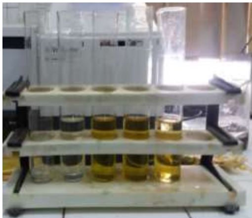
Fig5: Test of NH 3 using Nessler reagent.
